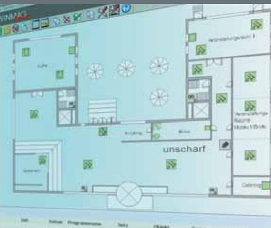
WINMAGLite, the hazard management system for one control unit, controls and visualises the most used functions of max. 1 fire, intrusion or access control system in combination with a CCTV system.
